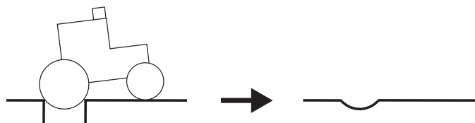
Figure 3.4: Partially unobservable true ground height due to wheel size
