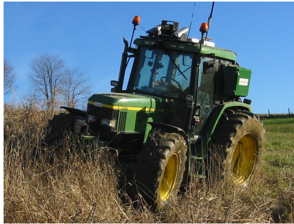
Figure 1.1: Automated tractor test platform (John Deere 6410)
