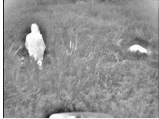
Figure 6.19: Infrared data showing high temperature of person and dirt mound
