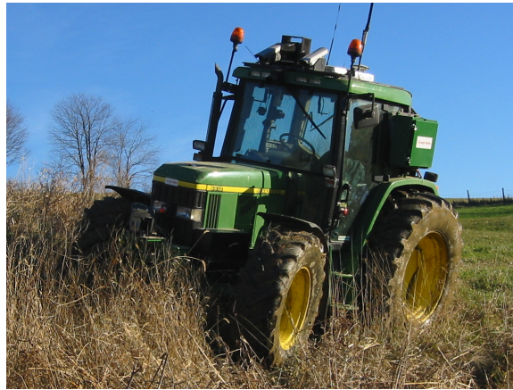
Figure 1.1: Automated tractor test platform (John Deere 6410)
